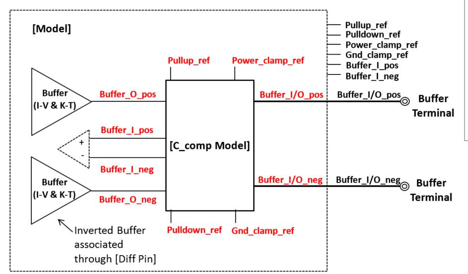
This C\_comp Model would allow direct RLC connections between buffer [Model]s, allowing for true differential buffer models.
